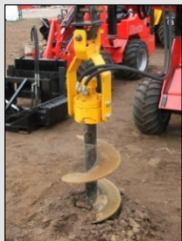
Earth drill installation
